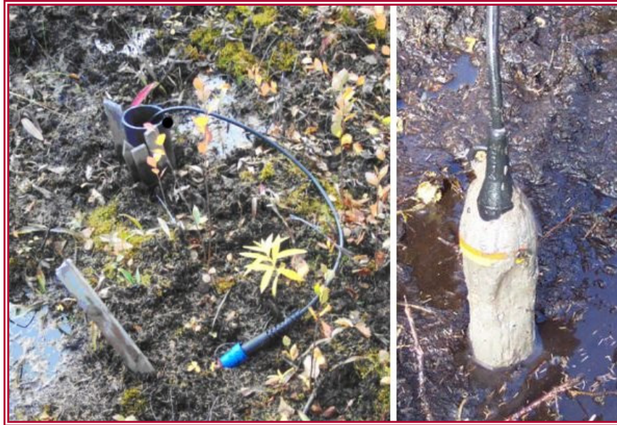
Figure 2. Deployment borehole for a subsurface receiver (left). Retrieved receiver seven months later, showing deployment in clay-mud in subsurface below muskeg (right).
