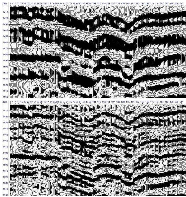
**Figure 3.** shows a segment of a seismic section from the input seismic data and the same segment from the reflectivity volume convolved with a bandpass wavelet with a high end of 120 Hz. Notice the higher resolution that has been achieved as well as the fact that lateral changes in wavelet character can now be studied. Data courtesy of Arcis Corporation, Calgary.
