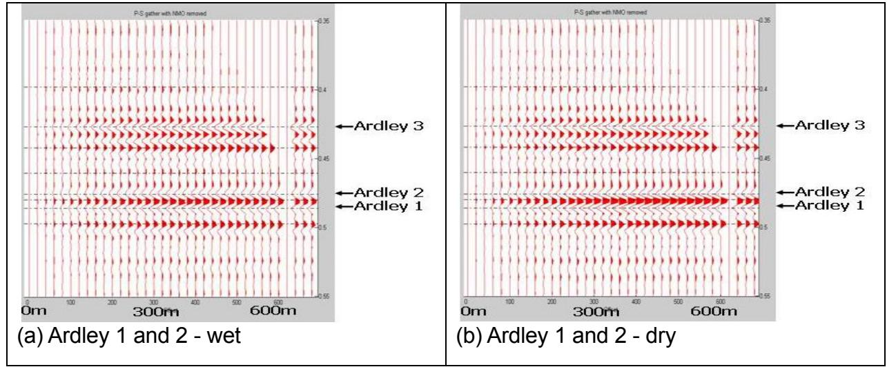
**Figure 3.** Synthetic offset gathers for PS reflections using a 90 Hz Ricker
