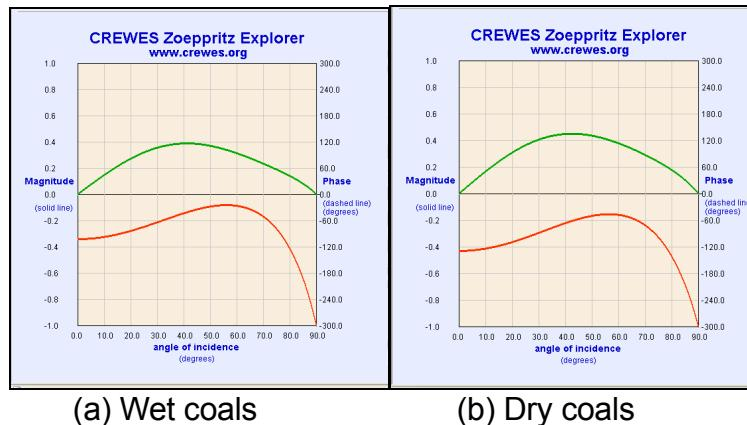
Figure 1. Reflection coefficients with angle of incidence for PP (red) and PS (green) waves at the top of Ardley 2.
