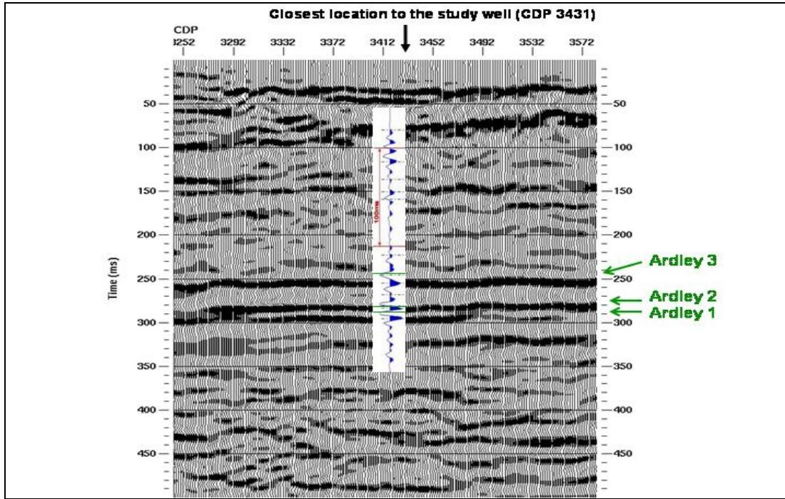
**Figure 4.** Migrated N-S seismic section with 90Hz Ricker synthetic tie
