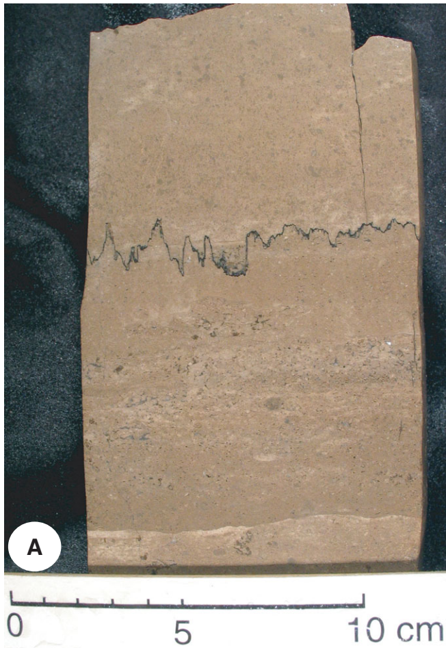
Figure 4. Lower Midale Beds. Limestones consist of a peloidal packstone. Development of stylolites and incipient solution seams define local diagenetic bedding in this facies (A). This facies shows considerable textural variability, including developments of a coarse-grained grainstone in parts (B). Peloids represent the predominant constituent, reflecting amounts between 60%-70%. Spar cement and porosity varies in amounts 15%-25% in average. Although skeletal fragments represent minor components, these packstones are characterized by a low-diversity body fossil assemblage, including calcareous algae, ostracods, foraminifera and undifferentiated material. Such a low-diversity assemblage of body fossils indicates deposition occurred in a relatively shallow-water, restricted lagoon environment.
