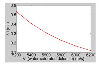
Figure 1: The effect of reservoir rock  $V_P$  on two-way traveltime differences resulting from fluid substitution.
