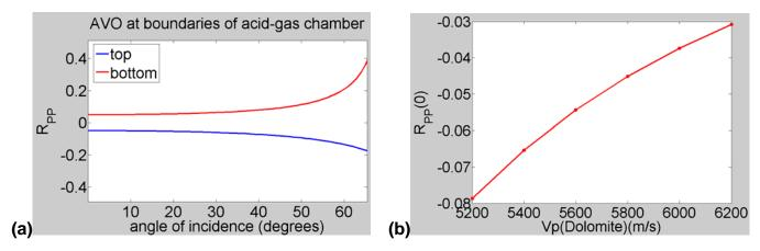
Figure 2: (a) Reflection coefficient curves defining RPP( $\theta$ ) at the top and bottom of an acid gas layer. The rock matrix is assumed to be constant across the interfaces, with brine saturation above and below the reservoir. (b) The effect of reservoir rock  $V_P$  on vertical reflectivity [ $R_{PP}(0)$ ] at the top of the injection chamber, given the same assumptions as in Figure 1.
