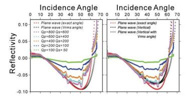
Figure 3: Scaled spherical-wave (numerical) reflection coefficients with constant Qp and Qs for top of layer 6 layers (Table 1). *Plane wave* denotes the same reflectivities calculated from Zoeppritz equation as in Figure 1.
