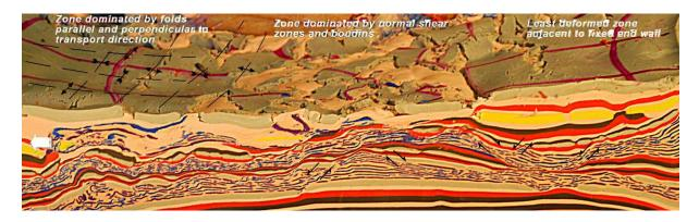
Figure 5: Oblique view of upper surface and vertical cut through a model simulating collapse between convergent lateral ramps showing changes from extensional to contractional deformation similar to that found in some deltas.
