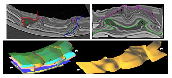
Figure 2: Top: CT scans parallel (left) and perpendicular (right) to the extension direction illustrate the geometry of silicone diapirs (tops in green and purple, right scan) and folds in adjacent intelayered modelling clay+silicone/silicone layers, and the deformation of early faults (red and blue). Bottom: gOcad reconstructions based on serial CT images of diapirs (gold) emplaced during dispacement on normal faults and a transfer fault.
