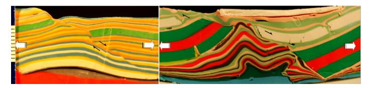
Figure 4: Folding of footwall and hanging wall layers during displacement on normal faults. The model at right comprises thick red and green competent and dense modelling clay layers, and lower modelling clay+silicone layers with a greater viscosity contrast in comparison to those in the left model. Ductile, less dense silicone (silver left, dark green right) separates basal and overlying layers.
