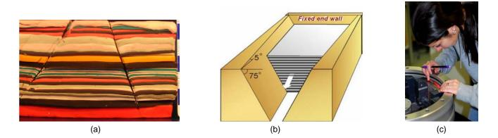
Figure 1: (a) Example of multilayered model prior to deformation where prescribed cuts represent faults. (b) Schematic diagram of lateral ramp models. Basal multilayers of modelling clay, silicone putty and modelling clay-silicone mixes were positioned between fixed wooden walls representing lateral ramps. Upper layers covered the entire base. (c) Models are positioned in the centrifuge rotor with layers vertical so that G forces act normal to initial layering.
