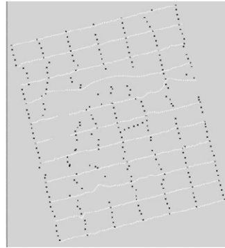
Figure 3: Moose Mountain 3-D survey layout. Dark circles are shotpoints and white lines are the receiver lines.
