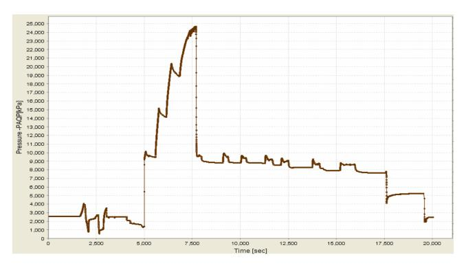
Figure3: Shale cap rock in situ stress test time/pressure results for SAGD cap rock in Western Canada.
