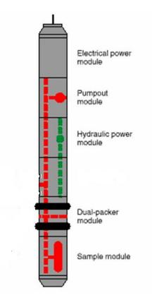
Figure1: Wireline stress testing tool configuration
