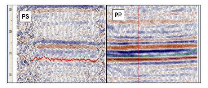
Figure 5: Comparison of the PS data (left) which has been stacked into an E-W 2D line and the comparable PP data (right) at the well location (red line). The Arbour/Mynheer Coal event is picked in red on the PS section.
