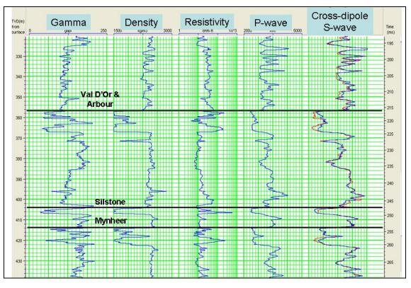
Figure1: Petrophysical logs from the injection well showing the Ardley Coal Zone
