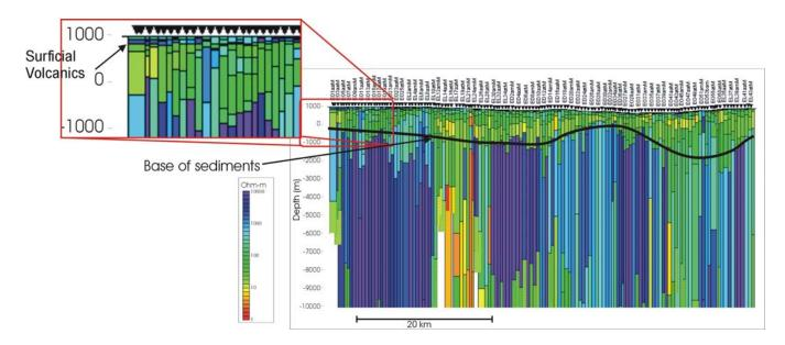
Figure 2: 1-D models for all of the sites as well as the surface geology along profile A. The warm colours represent conductive regions and the cooler colours resistive areas.
