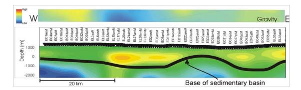
Figure 3: Stitched, smoothed 1-D models as well as gravity information along profile A. The conductivity colour scale is the same as that in figure 2.
