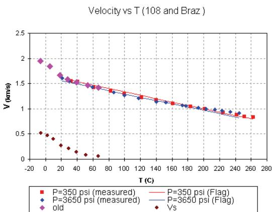
Figure 1: Measure Vp and Vs data versus temperature on two heavy oil samples.
