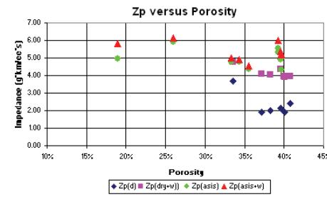
Figure 6: P-wave impedance versus porosity
