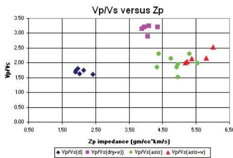
Figure 5: Measure  $V_p / V_s$  ratio versus P-wave impedance.
