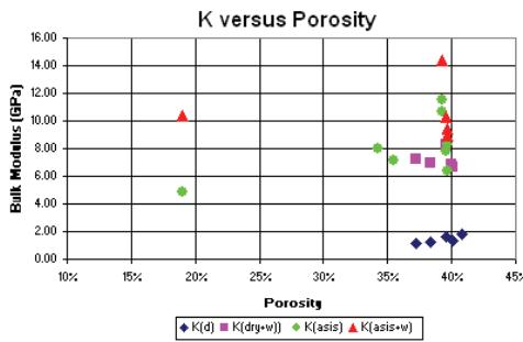
Figure 7: Bulk Modulus versus porosity
