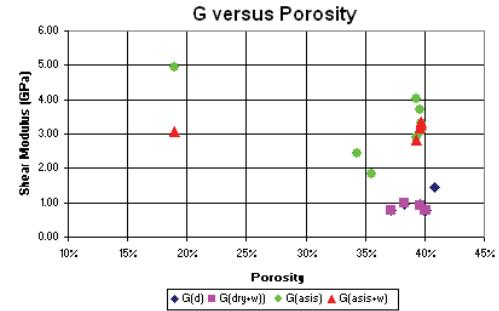
Figure 8: Shear modulus versus porosity
