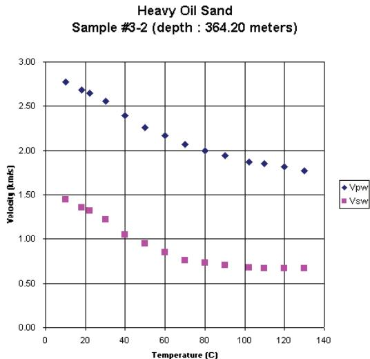
Figure 9: Measure Vp and Vs data versus temperature
