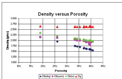
Figure 2: Measure bulk density, grain density and porosity.
