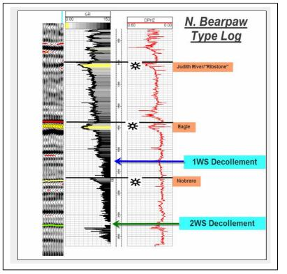
Figure 2: Type log for study area showing main gas reservoirs. Corresponding seismic section on left. Older 1WS decollement and younger 2WS decollement located in organic-rich shale.
