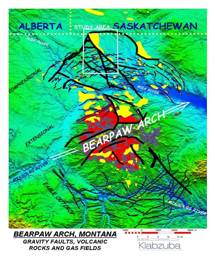
Figure 3: Bearpaw region DEM with gravity fault pattern in black. Faults south of the Bearpaws are exposed at the surface. Faults north of the Bearpaws are hidden beneath glacial veneer and have been mapped using seismic and well control. Eocene extrusive volcanics in red, intrusives in grey, and gas fields in yellow.
