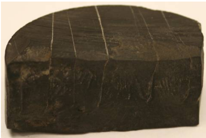
Core sample showing calcite-filled natural fractures
