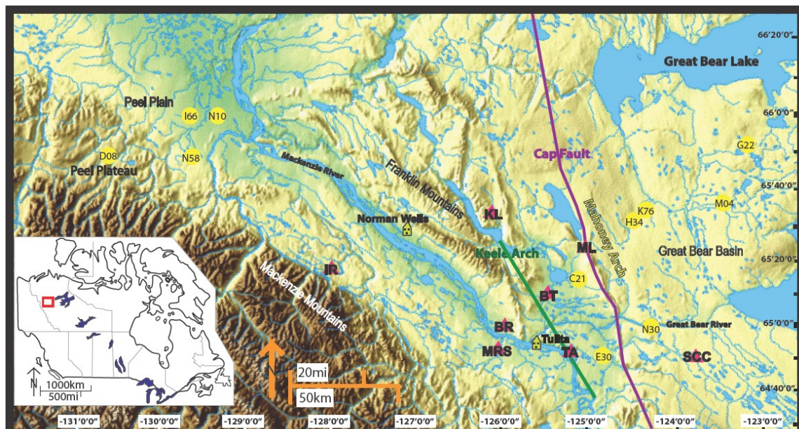
Figure 1 Map of the study area showing eleven cores (yellow circles), six measured outcrop sections (pink triangles), Norman Wells town (yellow house), Tulita community (yellow house). The Keele Arch (green line) is a reactivated fault structure, interpreted as a topographic high during the deposition of the Martin House Formation. The Cap Fault (purple line) was reactivated several times prior to the Cretaceous to form the Mahoney Arch. The base map is modified from the Department of Natural Resources Canada (2010).
