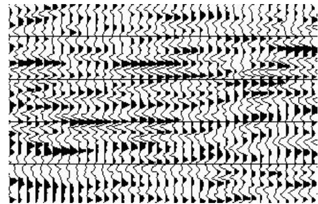
Figure 10: Unmigrated stack: FE rank 4 filter combined with C<sup>2</sup>-FX rank 2 filter on shots.
