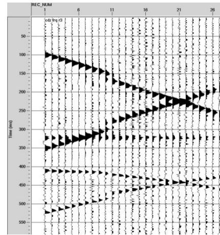
Figure 4: Difference plot: Input – FX Cadzow.
