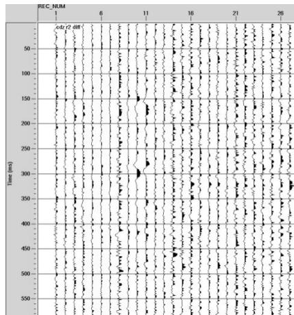
Figure 5: Difference plot: Input – FE filter.
