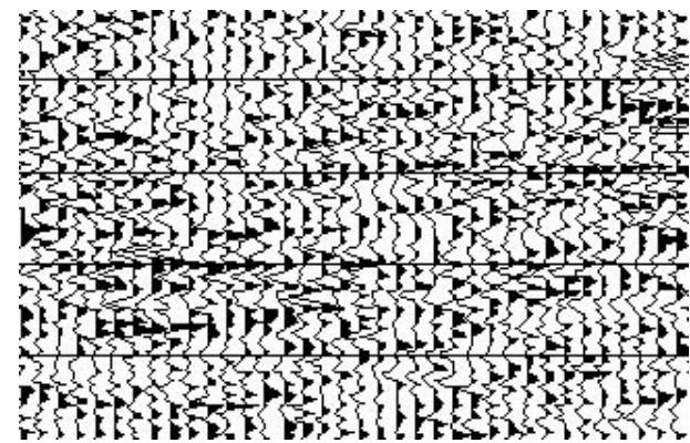
Figure 9: Unmigrated stack: C<sup>2</sup>-FX rank 2 filter on shots.
