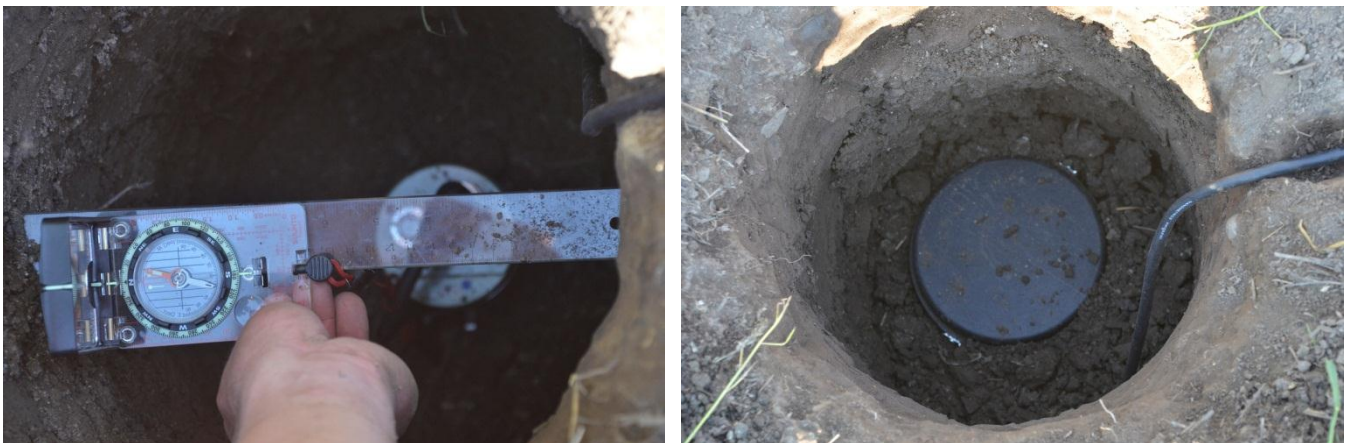
Figure 3: Shallow Posthole Installation
