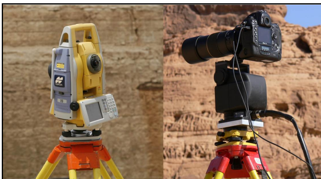
Figure 2. Topcon IS robotic total station on the left. FLIR pan-tilt robot with Nikon D3X
