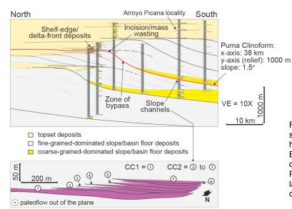
Figure 1. Overview of slope clinoform system in the Magallanes basin, highlighting the Puma Clinoform (from Bauer, 2012). Below, is a cross-section of slope channel complexes from the Petrel model. Channel complex 1 is labeled "1". The various channels of channel complex 2 are numbered 2-7.
