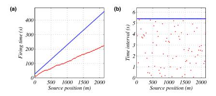
**Figure 1** Spatial and temporal distribution of firing time for conventional seismic acquisition (Blue) and 2D simultaneous source acquisition: one vessel scenario (red): a) Exact source Firing time of the whole acquisition b) Firing time intervals between adjacent sources
