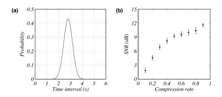
**Figure 4** Monte Carlo test with Binomial distribution: (a) Probability mass function of the firing time interval for  $\alpha = 0.5$ . (b) The SNR after deblending versus compression rate  $\alpha$ .
