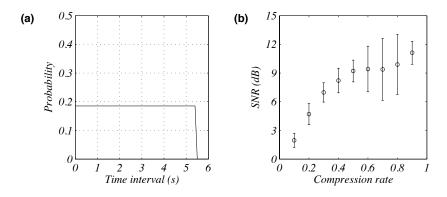
**Figure 2** Monte Carlo test with Uniform distribution: (a) Probability mass function of the random firing time interval for  $\alpha=0.5$ . (b) The SNR after deblending versus compression rate  $\alpha$ . The separation algorithm becomes unstable when the compression rate is around 0.7.
