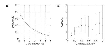
**Figure 3** Monte Carlo test with Exponential distribution: (a) Probability mass function of the firing time interval for  $\alpha=0.5$ . (b) The SNR after deblending versus compression rate  $\alpha$ .
