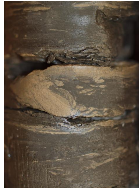
Fig. 4: Facies B, Thinly interbedded sandstone and mudstone displaying various sizes of load casts. Viking 3 reservoir unit, well 101/ 8-22- 30-25W3M
