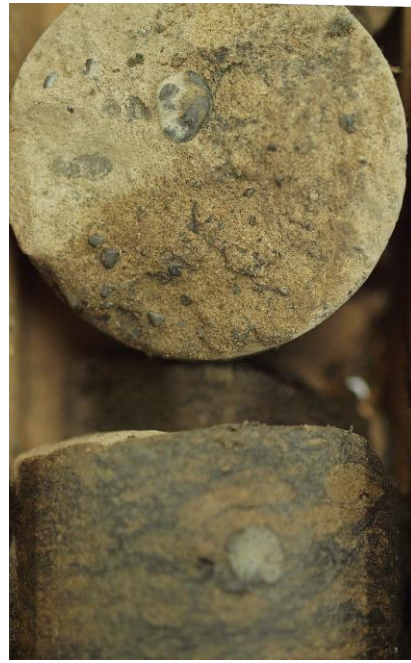
Figure 7: Facies D/Facies C Highly bioturbated medium grained sand of Facies C containing a large rounded chert clast abruptly overlain by a thin, fine-grained sandstone of Facies D at the base of a mudstone (Facies A). Contact between Viking 2 and 3, well 15-20-30-25W3M.
