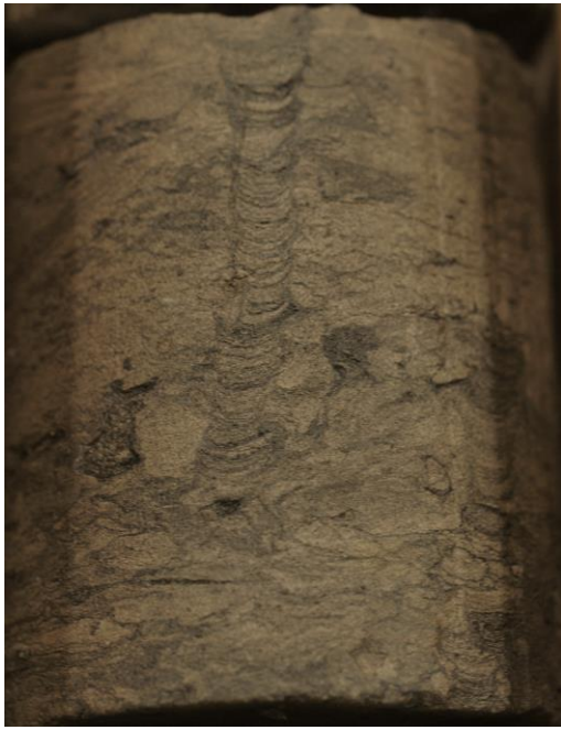
Figure 6: Facies C, highly bioturbated sandstone with primary bedding destroyed. Note the robust Teichichnus burrows. Viking 1 reservoir unit, well 101/12-31- 31-22W3M
