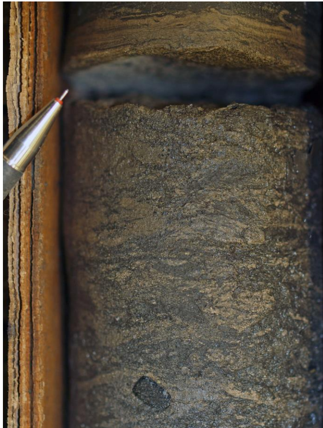
Figure 9: Highly bioturbated medium grained sandstone with scattered pebbles (Facies C) overlain by pebbles marking the base of Facies D. Contact between Viking 2 and 3 well 15-20?
